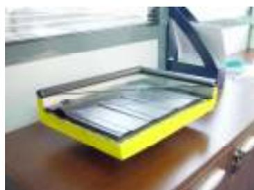
The use of polyurethane for the insulation of the flat plate collectors has 3 important benefits;
